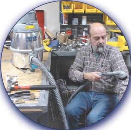
*GM 80 with brush attachment removes hazardous dust particles from clothing.*
