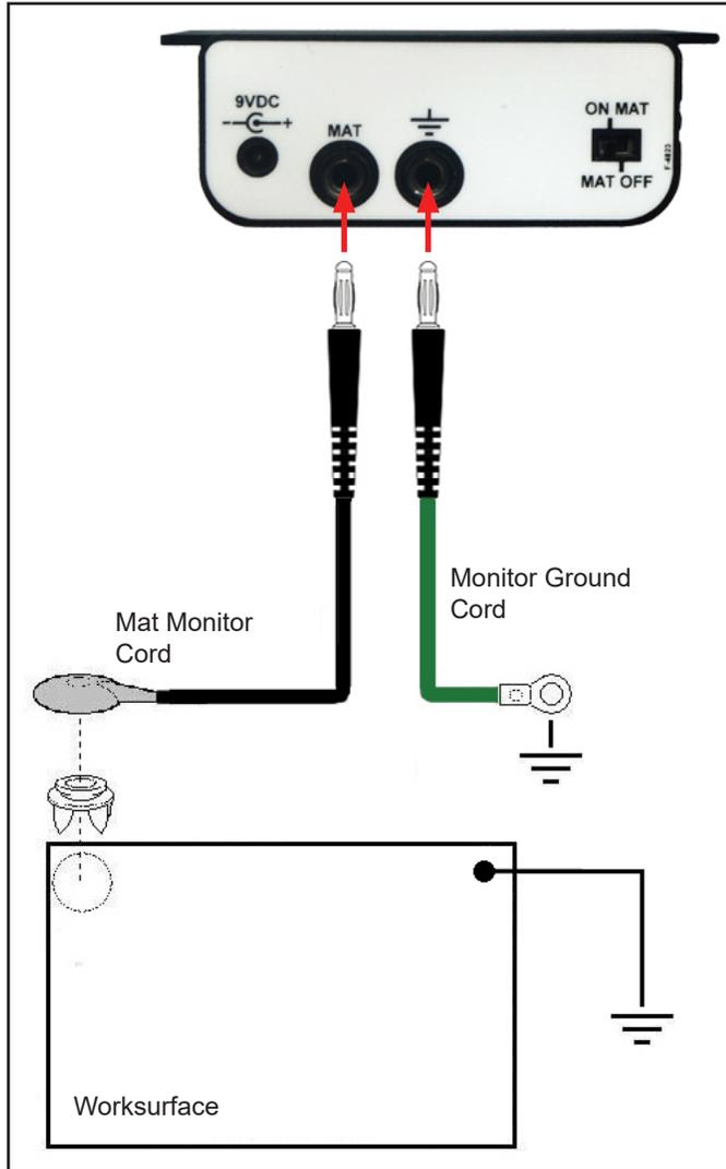
Figure 3. Installing the WSMONITOR2 Plus Workstation Monitor
