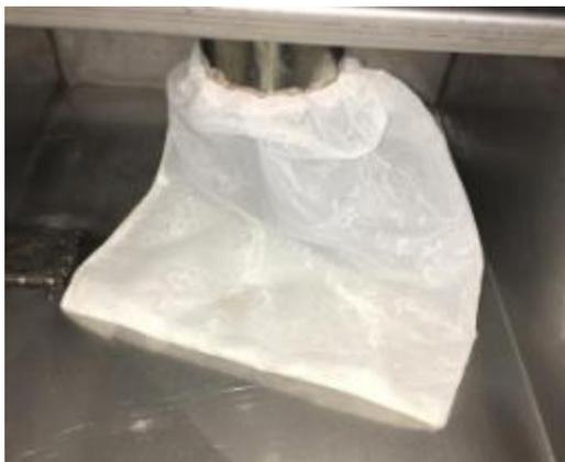
3.7 All 4 SUS304 stainless steel filters, filter tiny particles, filter precision  $5\mu\text{m}$  and  $1\mu\text{m}$ ;
