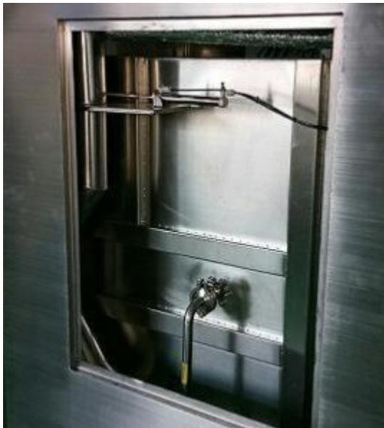
4.0. Detachable chute: convenient for maintenance, cleaning and maintenance;
